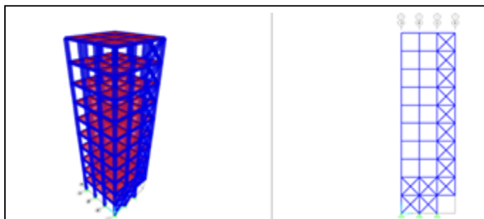
Figure 21: Floating column building provided with bracings at the corner on all storeys and the base
